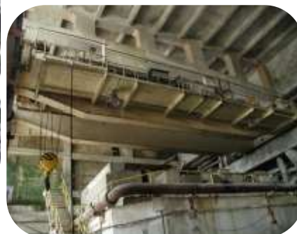
Gantry crane in a chemical facility was mechanically abraded and coated with Resichem 501 CRSG
