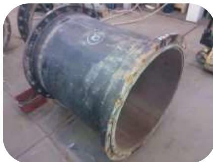
Pipe spool corroded from acidic water operating at 95°C was abrasive blast cleaned and coated with 206 HTA
