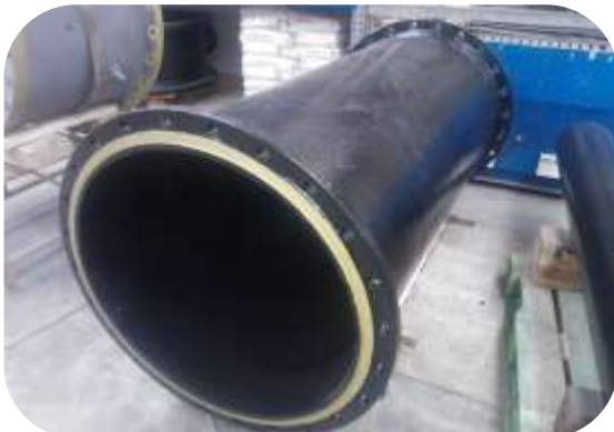
Pipe spool corroded from acidic water operating at 95°C was abrasive blast cleaned and coated with 206 HTA
