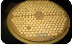
Badly pitted and corroded tube sheets and end plates can be rebuilt to original OEM specifications using 201 Ceramic Repair Paste
