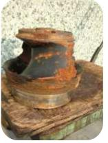
Chemical pump impeller had become badly corroded, the efficiency of the pump had been reduced by 50%. The impeller surface was abrasive blast cleaned and rebuilt using 201 Ceramic Repair Paste.
