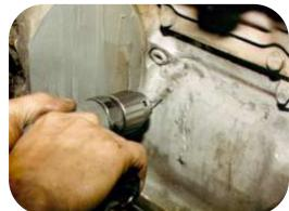
Emergency repair to a cracked engine block. The crack was drilled at both ends and then filled using 103 Metal Repair Stick
