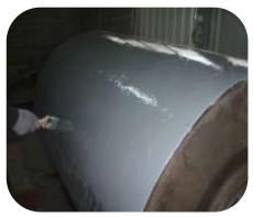
Conveyor belt roller prepared using needle guns and coated with 102 Metal Repair Fluid. Bauxite aggregate was incorporated into the wet resin to create an anti slip finish
