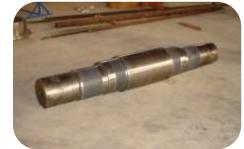
Shaft on stone crusher damaged and worn. Surfaces were rebuilt using 101 Metal Repair Paste and machined on a lathe to bring the shaft surface back to the original factory finish
