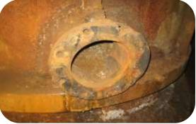
Damaged flange face repaired using 101 Metal Repair Paste
