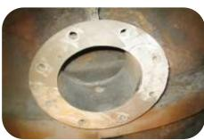
Corroded bow on large container vessel abrasive blast cleaned and filled using 101 Metal Repair Paste
