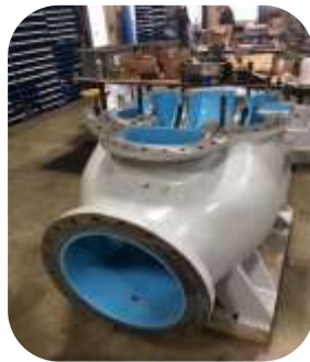
Large split case pump from a power station abrasive blast cleaned and then resurfaced using 203 Super Flow.
